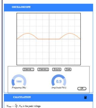
Ripple Factor= $\frac{V_{ac}}{V_{dc}}$  Since,  $V_{ac} = \sqrt{(V_{max}^2 - V_{dc}^2)}$
